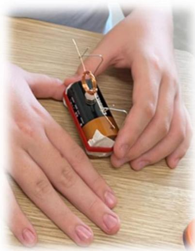
*Figure 2: Simple D-cell electric motor (Ethan)*
